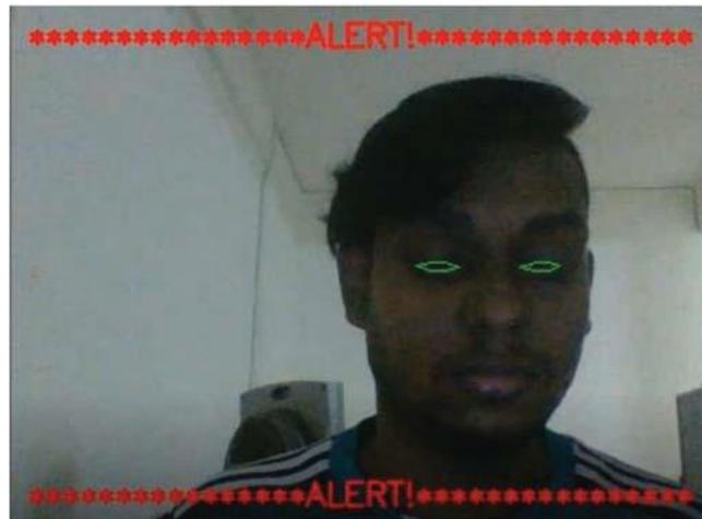
Fig. 9. Eye detection in dim light surrounding.
