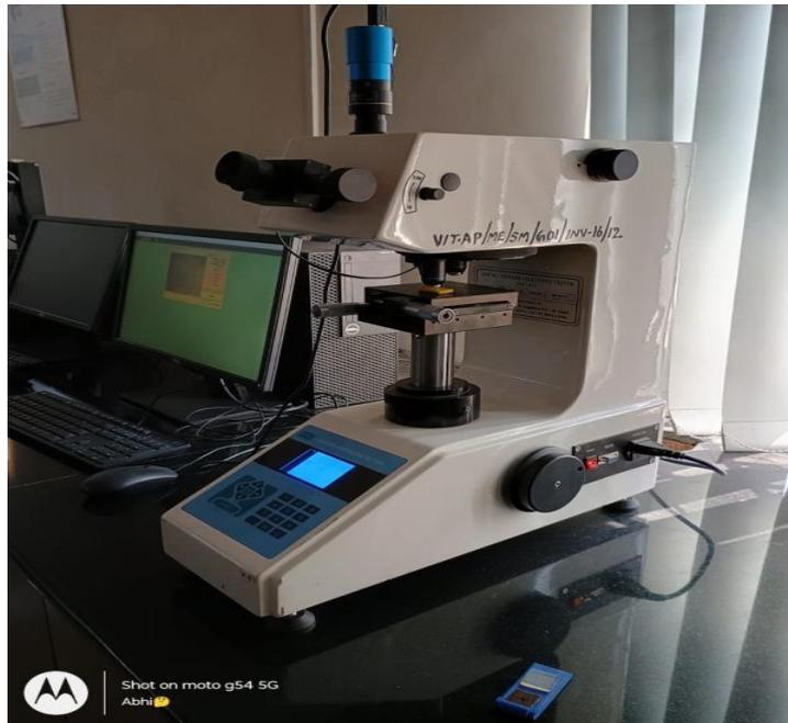
Prior to testing, specimens were carefully positioned on the testing stage as shown in figure 6, ensuring proper alignment and stability during indentation. The testing parameters, including the applied force and indentation duration, were set according to the ASTM E384 standard. In this study, a force of 100 grams force was applied to each specimen for a duration of 10 seconds, as specified by the standard.
