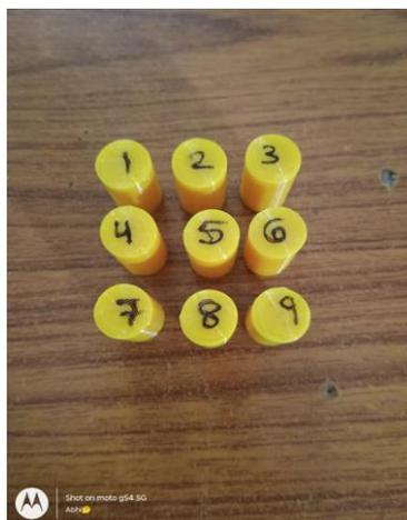
Figure 5: Compression Specimen Prepared from 3D Printer
