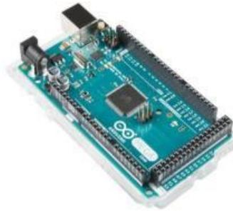
Figure 2 Arduino Mega 2560
