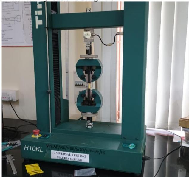
Figure 6: Tensile Specimen Placed in UTM
