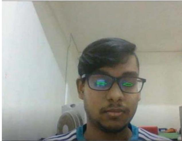
Fig. 8. Eye detection on wearing spectacles.
