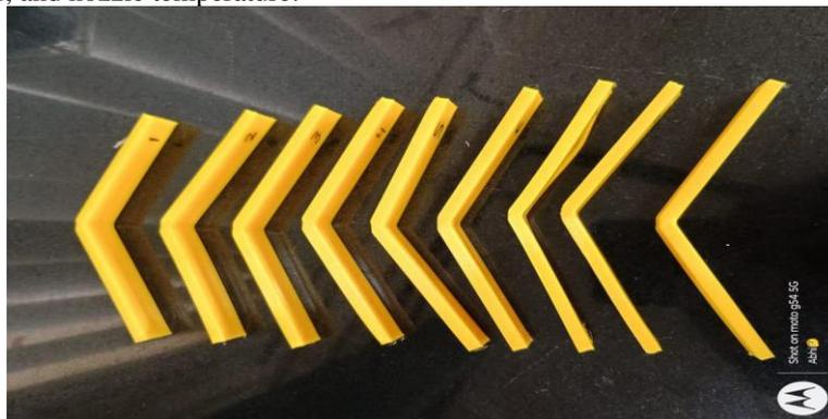
Figure 6: Flexural Specimens After Test
