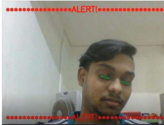
Fig. 10. Eye detection in microsleep condition.
