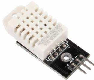
Fig.2 - DHT 22 Sensor (Temperature and Humidity Module)
