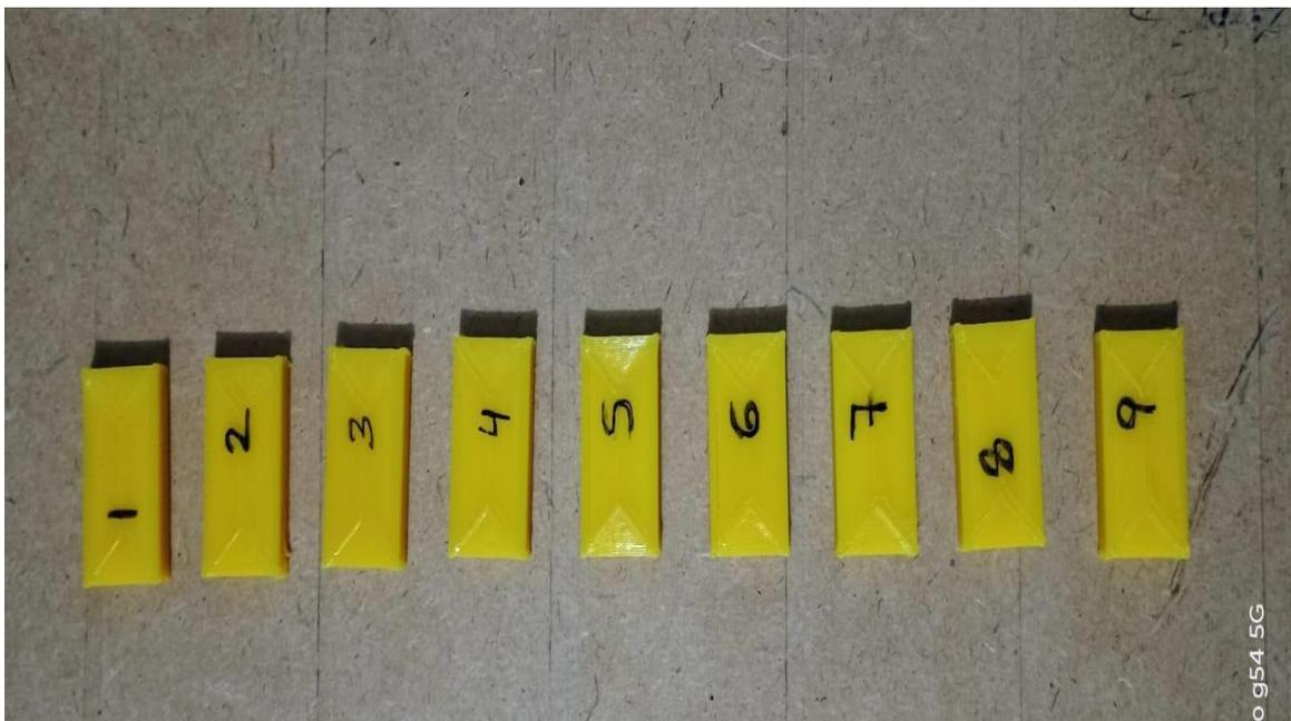
Figure 4: Hardness Specimen Prepared from 3D Printer
