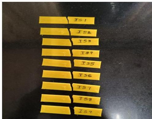
Figure 7: Impact Specimens After Izod Impact Test
