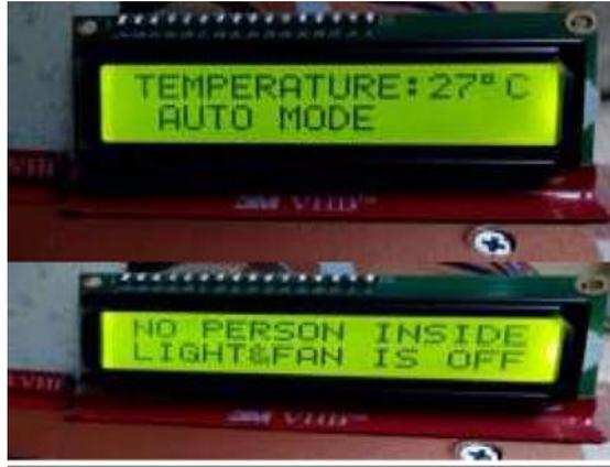
Fig.5: LCD displaying Automatic Mode
