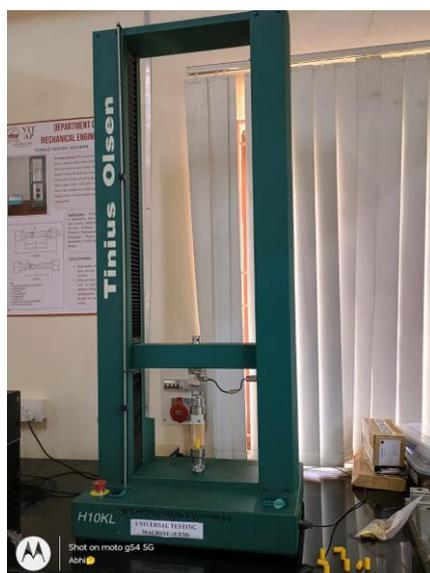
Figure 6: Compression Specimen Placed in UTM
